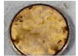
Figure 1 - Uncoated coin cell battery
